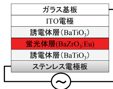
Fig.1 Double insulating structure of the EL device.
