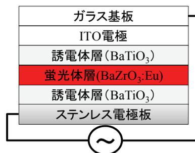
Fig.1 Double insulating structure of the EL device.
