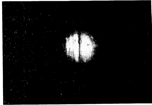
Fig. 2 Optical spot containing a line shadow on the screen.
