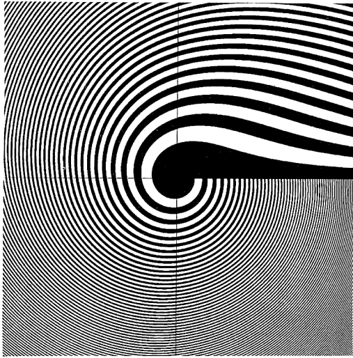
Fig. 2 Binary hologram mask for generating 2-D Fresnel zone plate, whose focal length is changed by rotation of masks.
