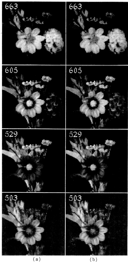
Fig. 4 (a) Cross sections of the original multispectral image that are perpendicular to the spectral axis. (b) Cross sections of the reconstructed multispectral image after the data compression by TSVQ. The number in each cross section denotes the wavelength.
