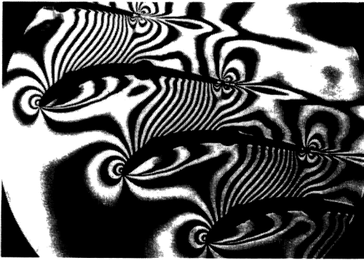
Fig. 1. Interferogram of pressure distribution around turbine blades.
