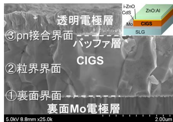
Fig. 1 Interfaces in a CIGS solar cell.
