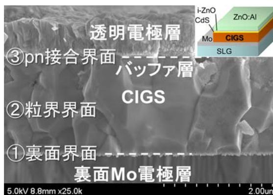
Fig. 1 Interfaces in a CIGS solar cell.
