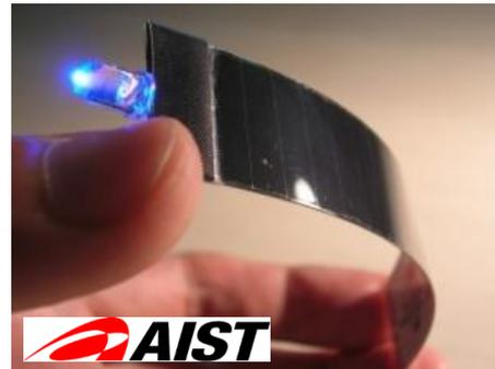
Fig. 2 Monolithically integrated flexible CIGS solar cell.
